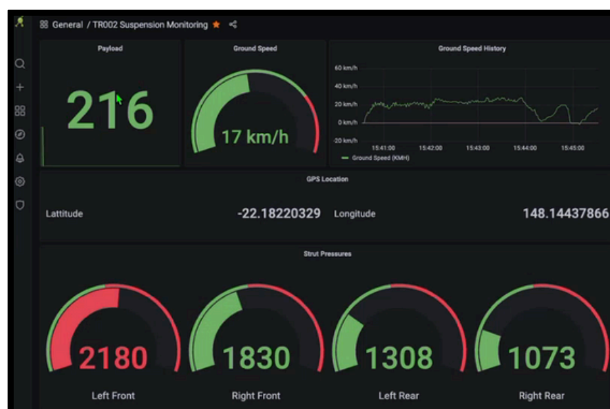
Figure 1: Data received for Suspension Monitoring of Mining Truck
